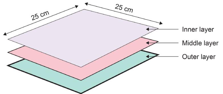
2. With the inner layer facing up, fold over 1 cm of the three pieces of material for the top and bottom edges and stitch at the borders (see red dotted lines).
